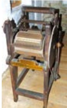
Arkwright's machine for "carding" cotton into yarn
